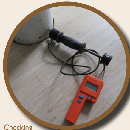
Checking the moisture content of a timber column using a resistance-type meter
