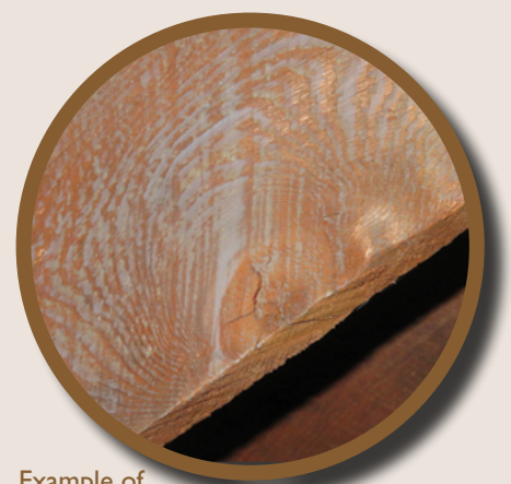
Example of an edge knot on a rafter
